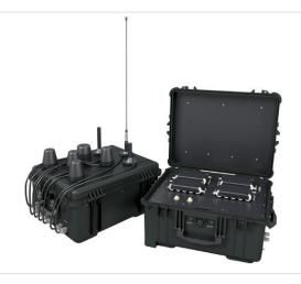
The CSU-3500W jammer is the universal solution for protection against RCIED threads that can be used as stationary, portable or vehicular system with communication windows setting.
